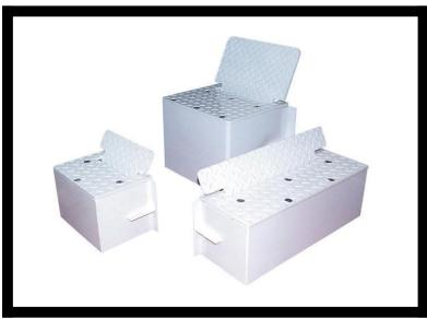
One-way Traffic Control Plates. For sinking into roadways to a depth of approximately 300mm. Drainage is required, also speed must be reduced to 5mph.
