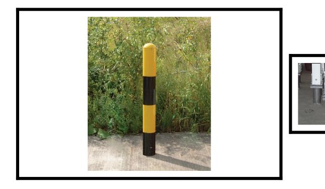
The Removable Domed Top bollard is made of a round mild steel tube. Tubular bollards have a slightly domed welded steel cap. The bollards are supplied galvanised as standard, and colour-coated finishes are available to order. The bollards can be used to protect buildings, shutter doors, etc., from accidental or deliberate vehicle impact.
