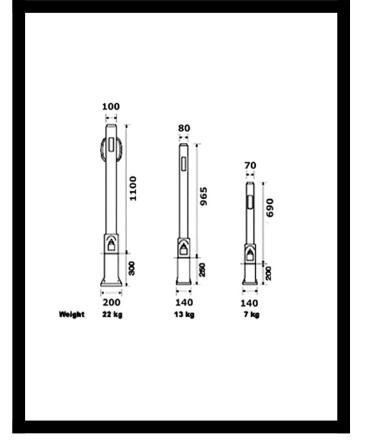
This range of bollards will meet all requirements to prevent un-authorised entry of vehicles and restrict access. The bollard is a heavy duty post that locates into a socket embedded into concrete. The post is locked in position by use of the socket flap and a padlock (not supplied). When the post is removed, the socket flap can be padlocked in the closed position keeping the socket free from rubbish until the post is next used.
