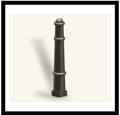
The use of Ferrocast bollards adds security to your landscape. These bollards are manufactured from engineering grade polyurethane which is cast around a steel core. This makes them virtually inert and the non-ferrous exterior means the bollard body will never rust, making them particularly suited to saline environments.
