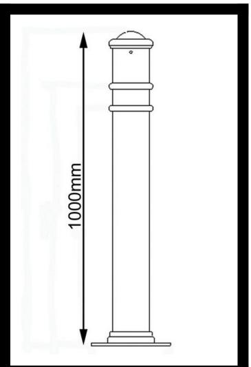
Fixed & Removable Ornamental bollards: Aesthetically pleasing, for safety, security and protection, preventing unauthorised parking and access. GFC ornamental bollards provide an attractive yet functional barrier to unauthorised vehicle access. This bollard is ideal for use around pedestrian precincts, pavements, play and parking areas, as part of traffic calming measures, pedestrianisation schemes and as a deterrent to ram-raiders.
