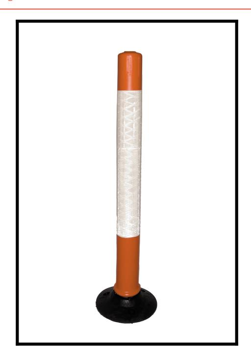
The link joint in the foot of the Flexible Post enables the cylinder to automatically return to the vertical position in the event of it being hit or run over many times. The base itself is manufactured from recycled material and can be secured by means of epoxy resin adhesive or single bolt fixing.
